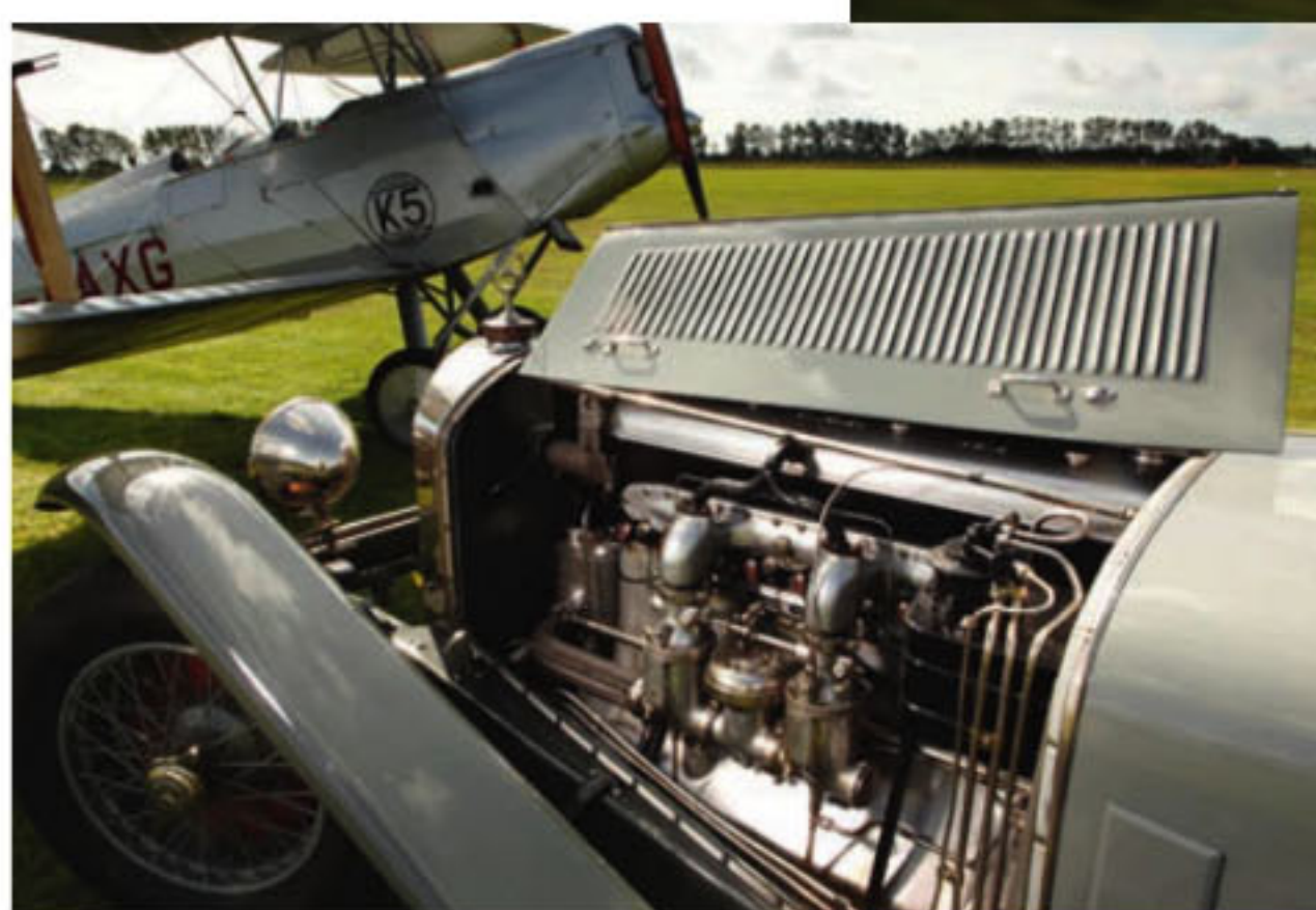
Clockwise, from top left: Moth, Mercedes and 'HK' (in cap) attract attention at Auckland Aerodrome in 1934; 6.7-litre sohc 'six' packs the engine bay; HK at the wheel of the car in single-seater form
