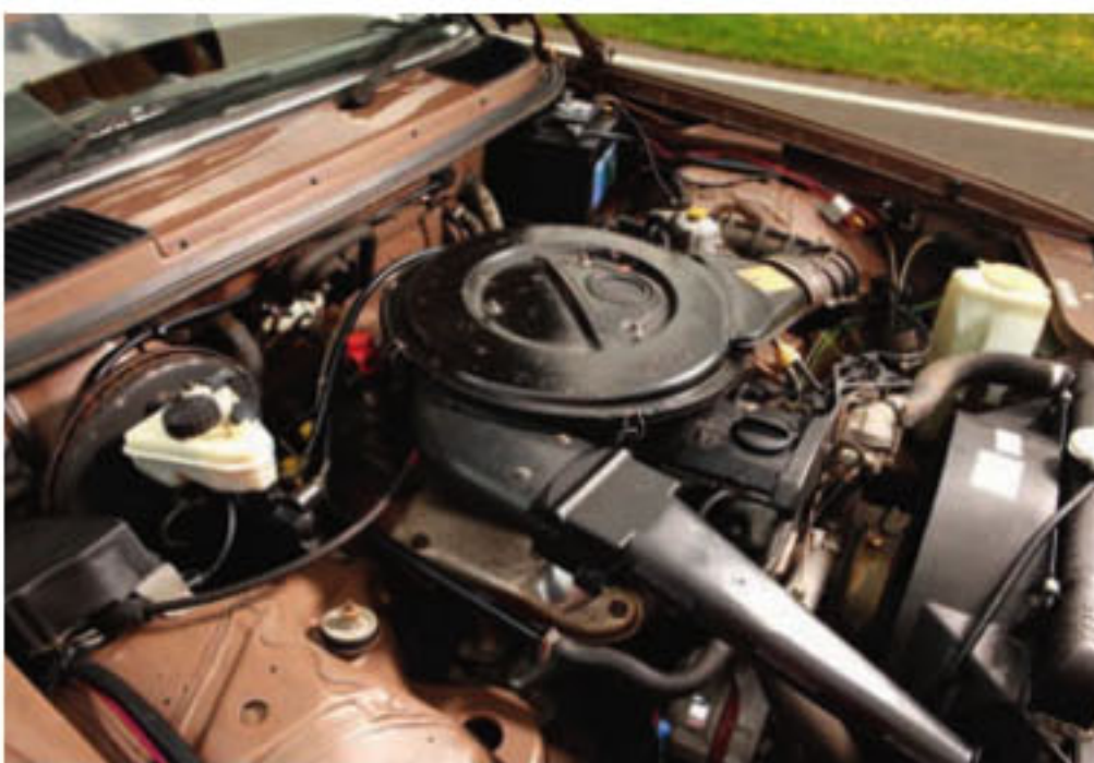
Crossflow head boosted entry-level 200 from 93 to 108bhp
