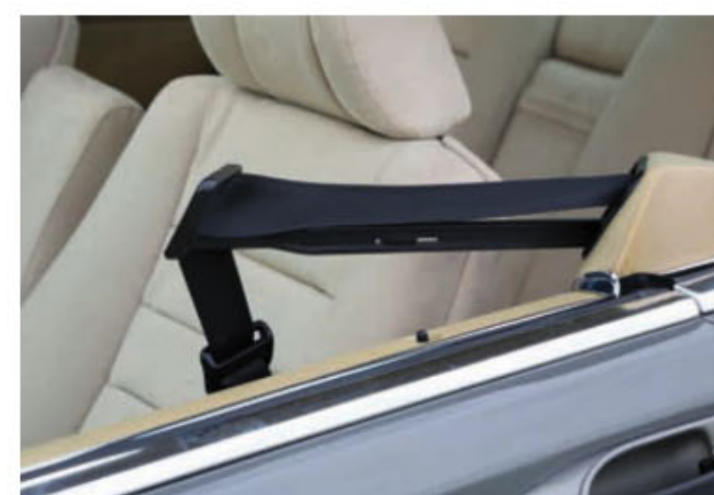
Clockwise: 560SEC is surefooted, with neat handling; seatbelts that extend automatically are among the model's high-tech gadgets; V8 develops a vast 325lb ft of torque, equating to effortless performance; airy cabin is beautifully finished
