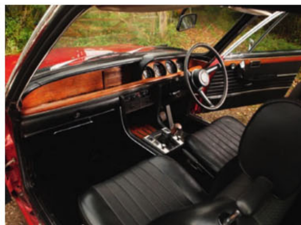
Fantastic all-round vision with slim pillars. Below, l-r: injection raised output of 3-litre M30 'six' by 20bhp; 195/70s on factory 14in alloys; sculpted seats, but least roomy of four; trim is vinyl (usually velour)
