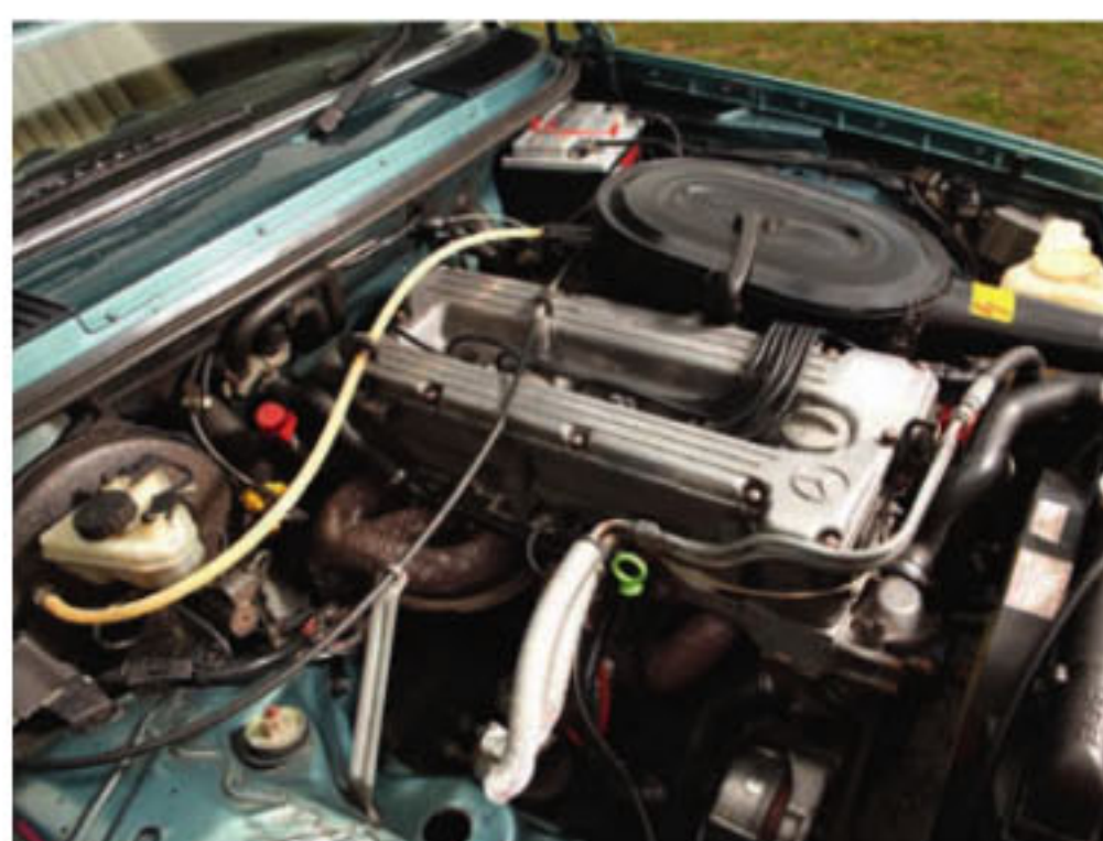
Fuel-injected twin-cam 2.8 offers a free-revving 182bhp
