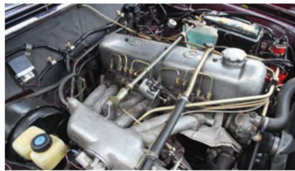
Rebuilt 2.2 straight-six now runs 123 electronic ignition
