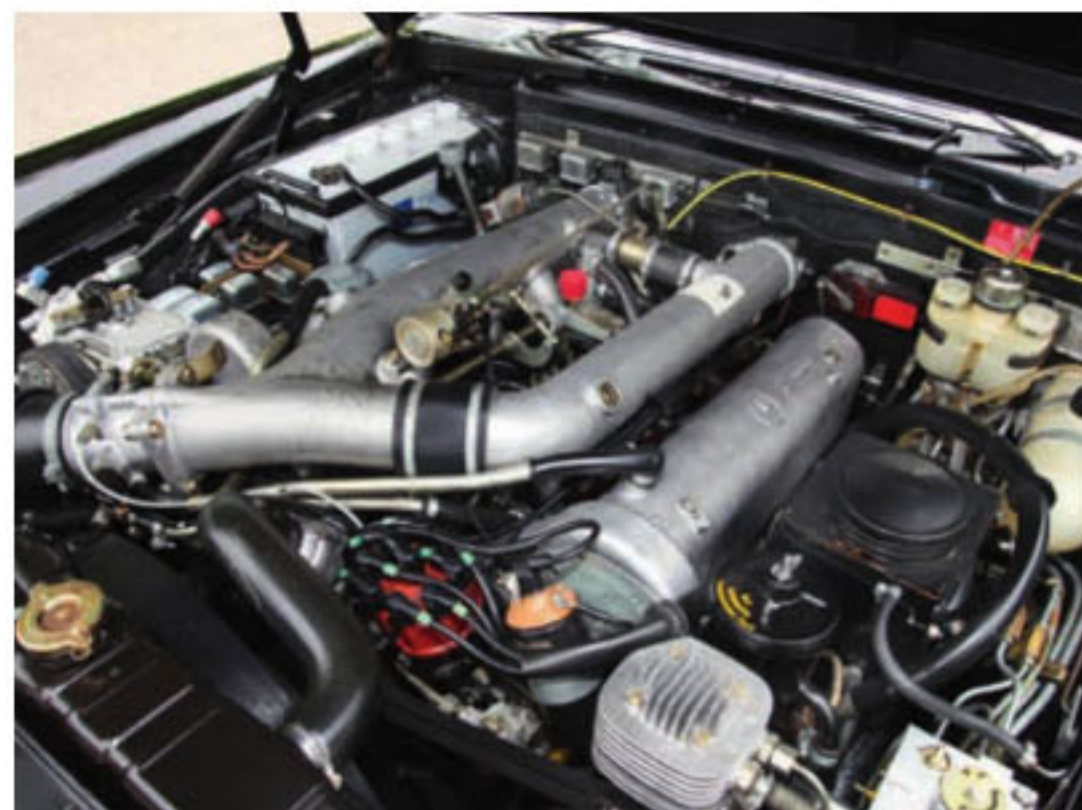
M100 motor has seven auxiliary drives off its crank pulley, including two alternators to feed its electrical demands
