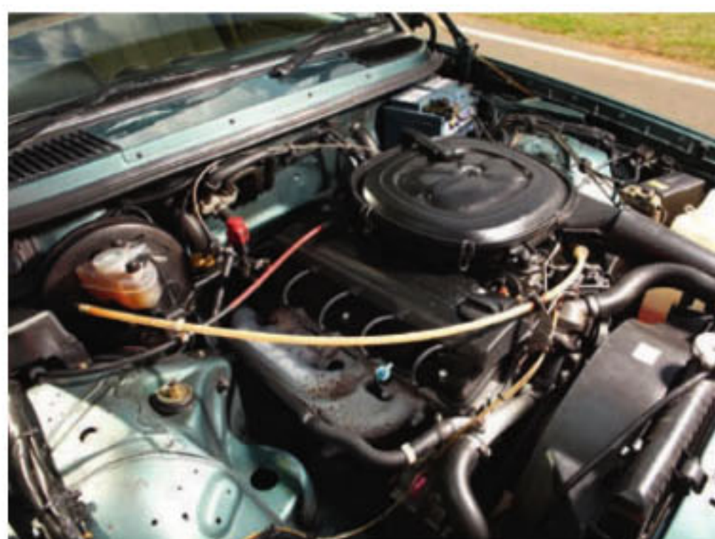
Peppy injected 2.3 produces 134bhp and 148lb ft of torque
