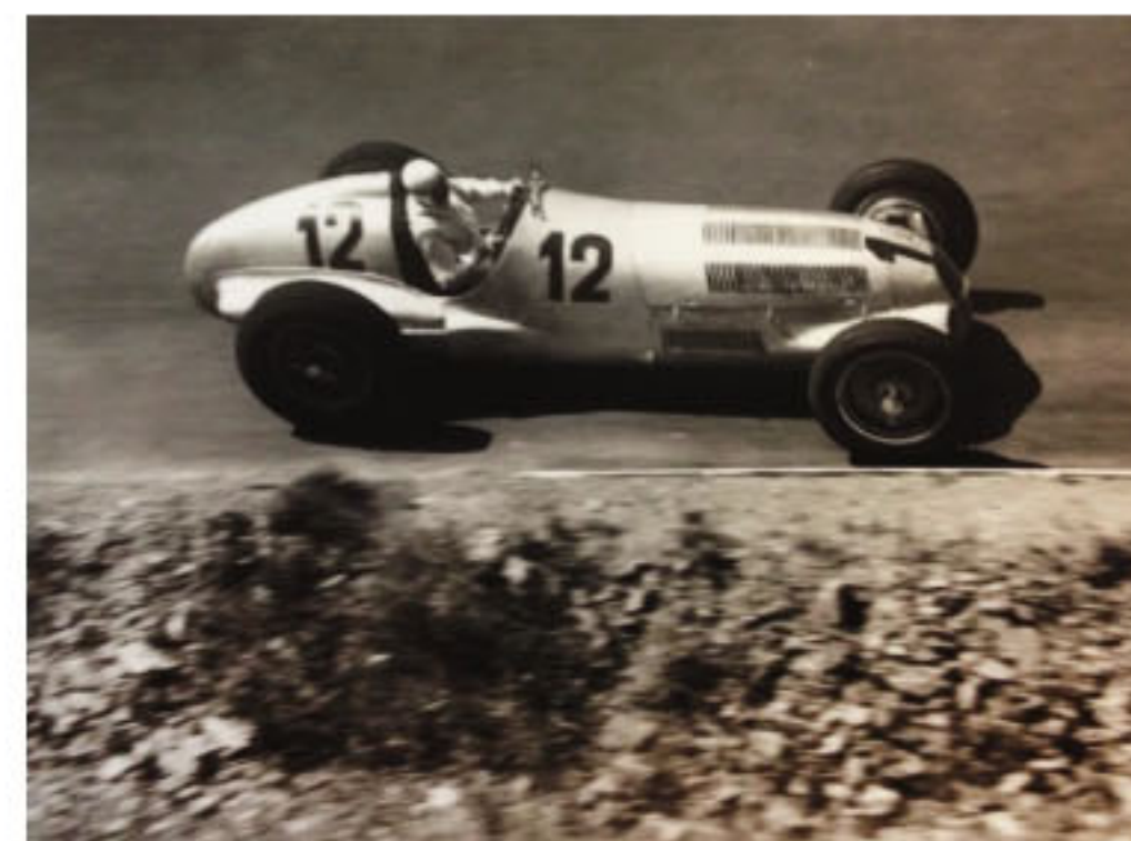
Below: Caracciola en route to victory in German GP; slick four-speed gearbox is largely redundant with 632lb ft peak torque developed at just 3000rpm
